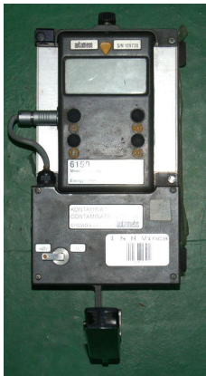
Automess 6150 AD contamination probe
